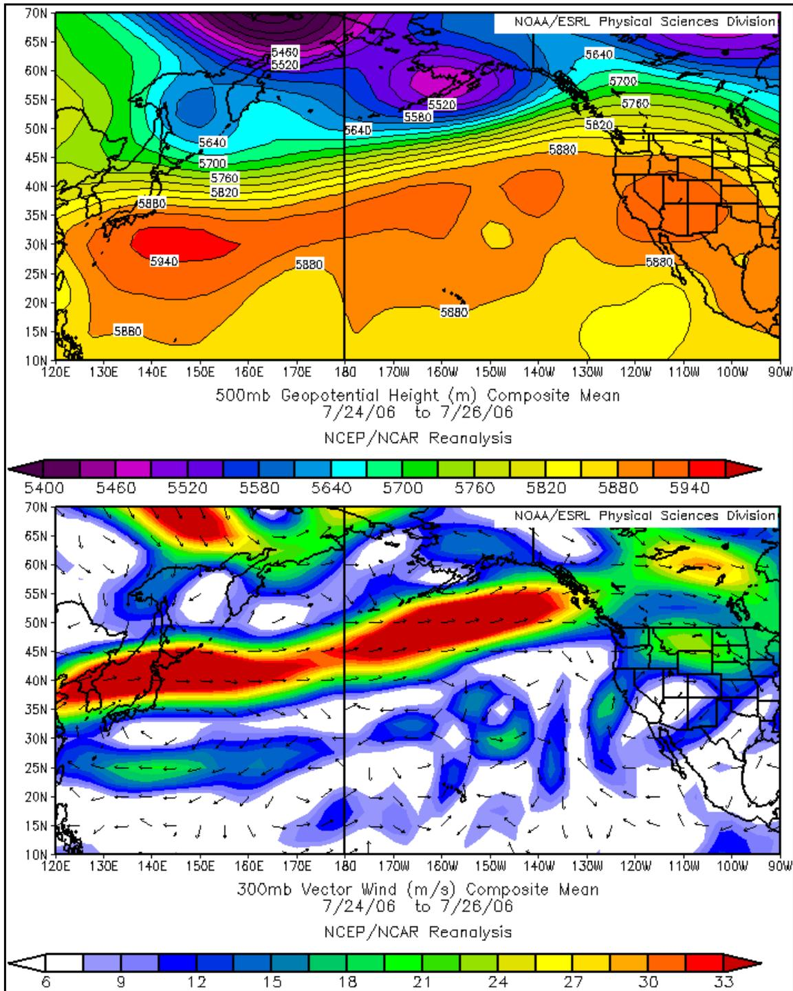
**Figure 7:** Indicates the 500mb geopotential heights (m) and 300mb vector wind (m/s) from July 24 through July 26, 2006. This shows the increasing heights across the east-central Pacific, as well as the strengthening zonal jet stream crossing the Pacific. This zonal jet stream reduced the amplified flow, including the western United States upper level high pressure ridge responsible for the July 2006 heat wave.
