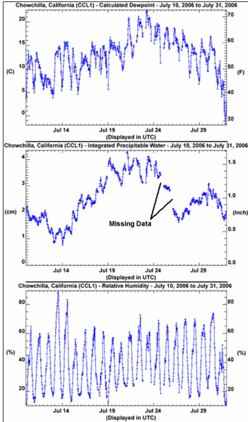
**Figure 16:** Depicts three unique moisture parameters, surface dew point temperature, integrated precipitable water, and relative humidity at Chowchilla, California (north-central San Joaquin Valley) from July 10 through July 31. Notice the increase of surface dew point temperature and integrated precipitable water values during the peak of the heat wave event. Also, notice the lack of change in relative humidity, except for typical diurnal fluctuations.
